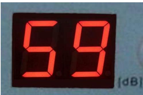
When not using Smart Mode, you can manually lower your repeaters gain by adding attenuation. Every press on the - or + button will manually decrease (or increase) the total gain by 1 dB. You can manually decrease gain from 70/75 down to 36/41dB.
